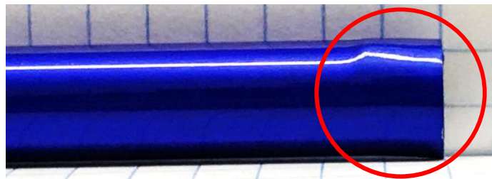
Fig. 14. Plastically deformed barrel at the larger diameter end, where the cap press-fits.
