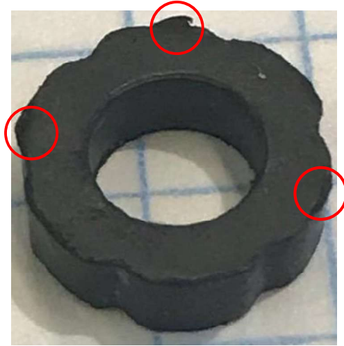
Fig. 10. A completed pressure gauge washer with red circles identifying excess material along the edges.
