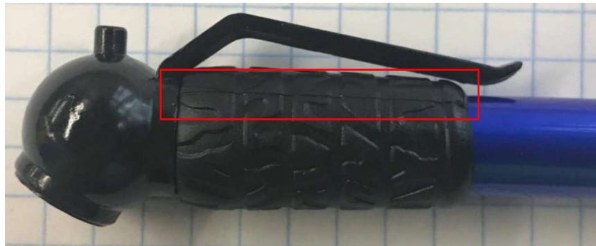
Fig. 12. Detailed view of flash along the grip's outer surface from the injection molding process.
