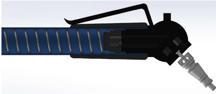
Fig. 2. Detailed view of the pressure gauge interacting with a Schrader valve
