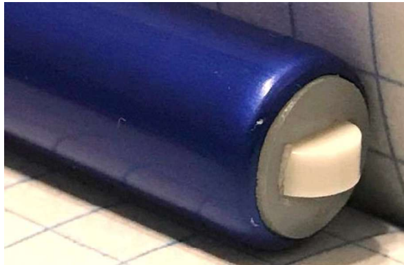
Fig. 16. Barrel's filleted edge along its smaller diameter, housing the keeper and the ruler.
